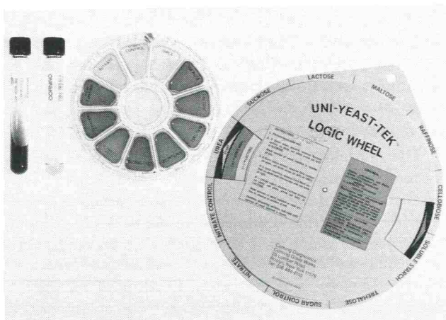
Figure 23. Uni-Yeast-Tek . A system to identify yeast. With permission from Corning Medical Diagnostics, Corning, NY.
