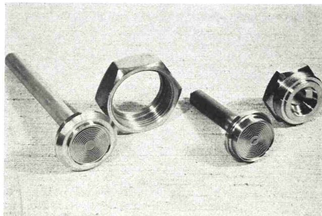
Figure 2. Typical sanitary (left) and non-sanitary volumetric pressure elements.
