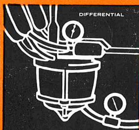
Two separate vacuum systems, one for pulsators . . . one for the milk line. Reports say, "Production goes up . . . udder health improved."
