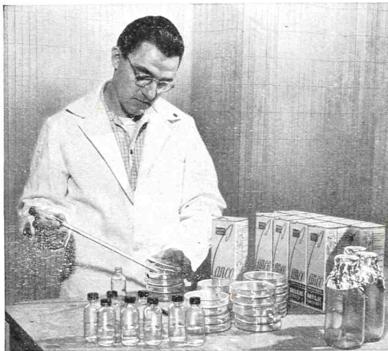
Frequent rinse tests in accordance with standard methods for the examination of dairy products are made at Canco factories to keep a continuing check on compliance with the Public Health Code. Photo shows Canco technician transferring rinse solution from containers to sterile Petri dishes.
