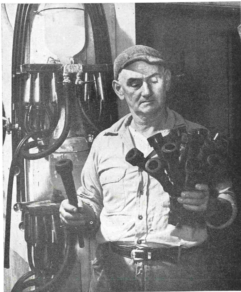
This farmer discarded 15 rubber inflations but only one neoprene inflation during ten months of tests. Each of his units was equipped with two rubber and two neoprene inflations.
