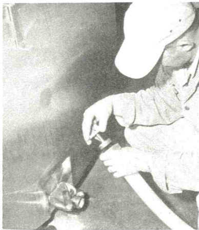
Cap used to seal off end of Tygon tubing. During pump-out operation, cap is placed on floor in inverted position so that sanitary threads do not touch floor.
