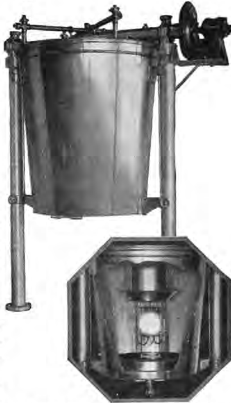
The CP Milk Irradiator. Inset shows part of drum cut away to give a better view of the carbon arc lamp.
